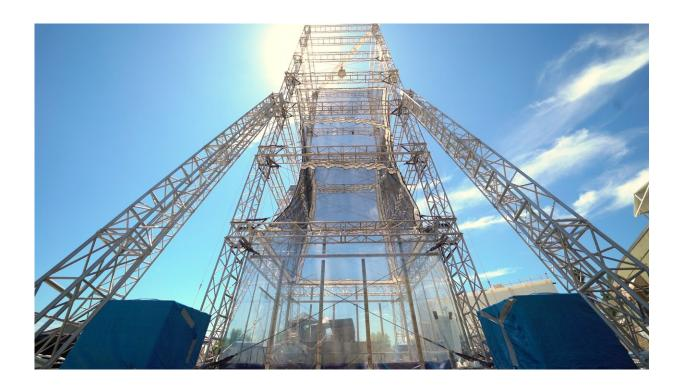
This drop tower at JPL includes a bow launch system, which can hurl test articles 110 mph into the ground, re-creating the forces they would experience during a Mars landing. Credit: NASA/JPL-Caltech
