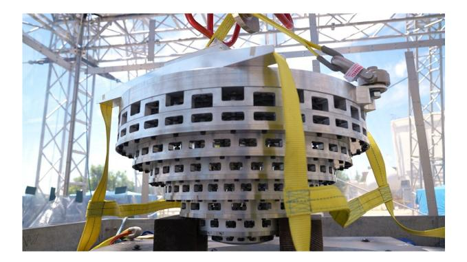
This prototype base for SHIELD – a collapsible Mars lander that would enable a
