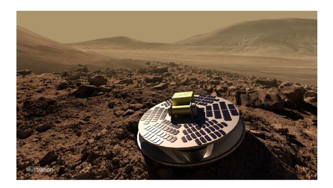
An illustration of SHIELD, a Mars lander concept that would allow lower-cost missions to reach the Red Planet's surface by safely crash landing, using a collapsible base to absorb the impact. Credit: California Academy of Sciences
