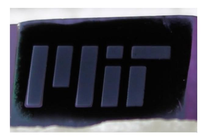
Caption: MIT engineers fabricate a forest of "white graphene" nanotubes (shown here patterned as MIT) by burning away a scaffold of black carbon. Credit: the researchers
