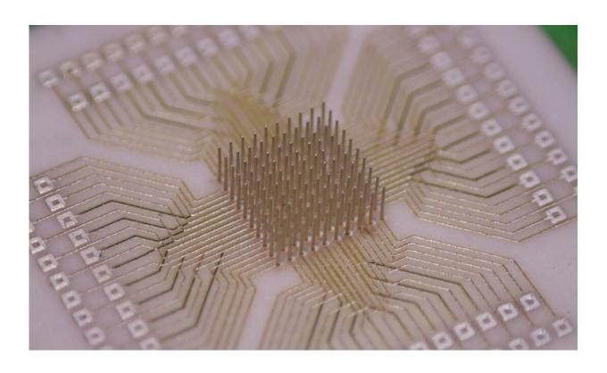
Researchers used Aerosol Jet 3D printing to produce a new type of microelectrode array that solves the major design barriers of other brain computer interface arrays. Credit: College of Engineering Carnegie Mellon University
