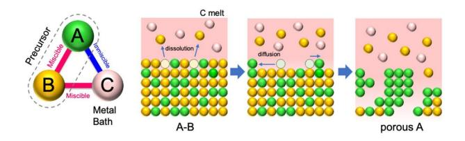
The principle and self-organizing process of liquid metal dealloying. In the precursor alloy (AB), the pore-forming metal (A) and sacrificial component (B) should have a positive and negative enthalpy when mixing with the melt bath (C), respectively. With the component B selectively dissolving into C melt, the remaining component A self-organizes into a porous structure. Credit: Takeshi Wada and Ruirui Song
