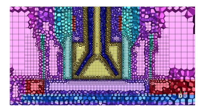
Computational grid for thermal simulation with a magnified representation of the NanoCube exposure device. The aerosol sections are in yellow, the other sections are either components or air sections. Credit: Fraunhofer SCAI
