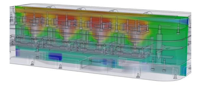
A snapshot of the simulation shows the temperature distribution in the NanoCube with the multi-organ chips inside. The analysis of the temperature distribution helps to improve the design of the NanoCube. Credit: Fraunhofer SCAI
