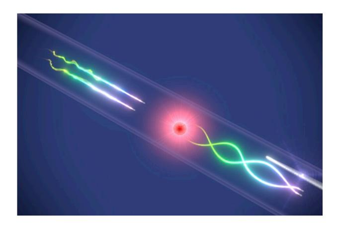
Two photons propagating in a waveguide interacting with a single quantum emitter. The photon-photon interaction, which results in correlations. Credit: Le Jeannic et al.
