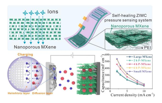
The design of nanoscale ion channels, MXene electrodes with maximized ion accessibility and high mechanical strength are constructed and used for high-capacity Zinc-ion energy storage. The design of in-plane ion channels provides a simple, efficient and scalable approach to effectively improve the electrochemical energy storage capacity of MXenes and other 2D materials. Credit: Science China Press
