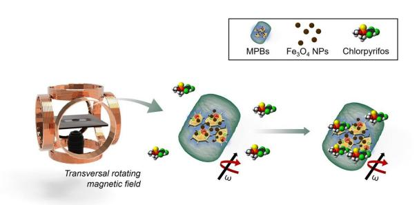
Schematic illustration of chlorpyrifos removal by propelled magnetic plant biobots (MPBs) under a transversal rotating magnetic field. Credit: *NPG Asia Materials* (2022). DOI: 10.1038/s41427-022-00425-0
