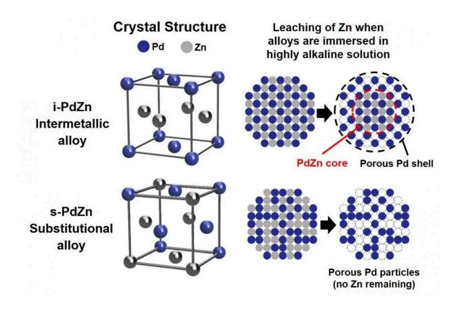
The crystal structure of the intermetallic i-PdZn alloy allows Zn to be retained at the core, surrounded by a protective shell of Pd atoms. This gives the i-PdZn better corrosion resistance when immersed in highly alkaline solutions, unlike the substitutional alloy s-PdZn, where random replacement of Pd atoms by Zn in the crystal structure allows the Zn to leach out quickly. Credit: Hiroshi Inoue, Osaka Metropolitan University
