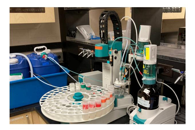
Robotitrator that is used to measure alkalinity of the water. Image courtesy of Hannah Hensel. Credit: Hannah Hensel
