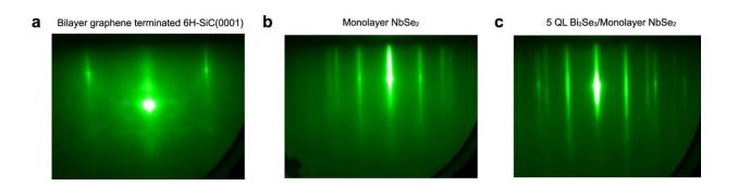
RHEED patterns during MBE growth. (a) Bilayer graphene terminated 6H-SiC(0001) substrate. (b) Monolayer NbSe<sub>2</sub> film grown on bilayer graphene. (c) 5 QL Bi<sub>2</sub>Se<sub>3</sub>/monolayer NbSe<sub>2</sub> heterostructure grown on bilayer graphene. Credit: *Nature Materials* (2022). DOI: 10.1038/s41563-022-01386-z
