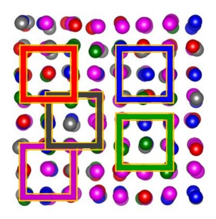
The Cantor alloy under study consists of chromium (gray), manganese (pink), iron (red), cobalt (blue), and nickel (green). X-ray methods allow to probe each individual component in an element-specific way. Credit: A. Kuzmin/University of Latvia and A. Smekhova/HZB
