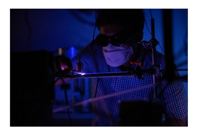
A ray of plasma, which glows pink, is used to activate a gas of hydrogen and methane molecules and break them down into smaller fragments. The sample to be coated, such as a two-dimensional copper line, is then immersed in the plasma, and carbon from the gas gets deposited onto the surface as thin sheets of graphene. Credit: Caltech
