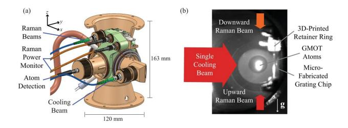
Concept of the compact light-pulse atom interferometer (LPAI) for high-dynamic conditions. **a** 3D rendering of the compact LPAI sensor head with fixed optical components and reliable optomechanical design. **b** Picture of the steady-state GMOT atoms in the sensor head.. Credit: *Nature Communications* (2022). DOI: 10.1038/s41467-022-31410-4
