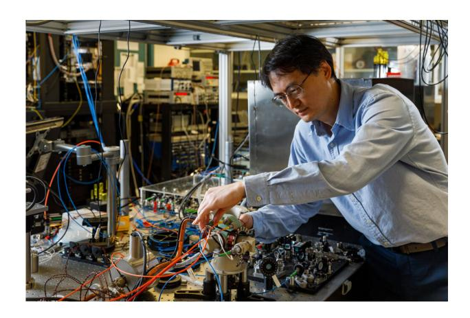
Sandia atomic physicist Jongmin Lee examines the sensor head of a cold-atom interferometer that could help vehicles stay on course where GPS is unavailable. Credit: Bret Latter
