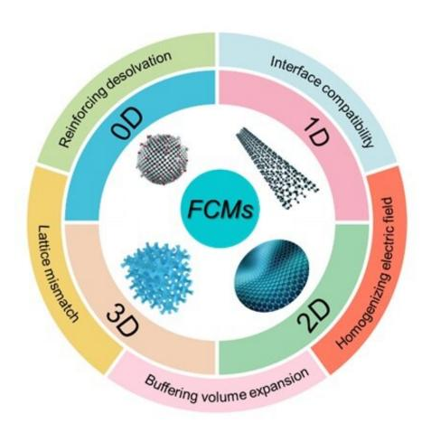
Functional carbon materials addressing dendrite problems in metal batteries: surface chemistry, multi-dimensional structure engineering, and defect. Credit: Science China Press
