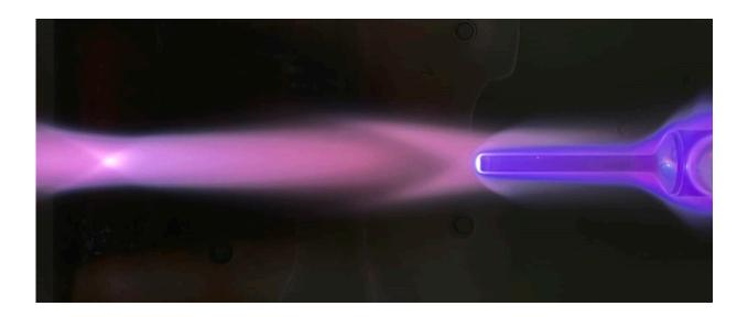
Enthalpy probe in the supersonic plasma jet is used to measure flight conditions—including pressure and heat –simulated in the tunnel. Credit: University of Illinois Dept. of Aerospace Engineering
