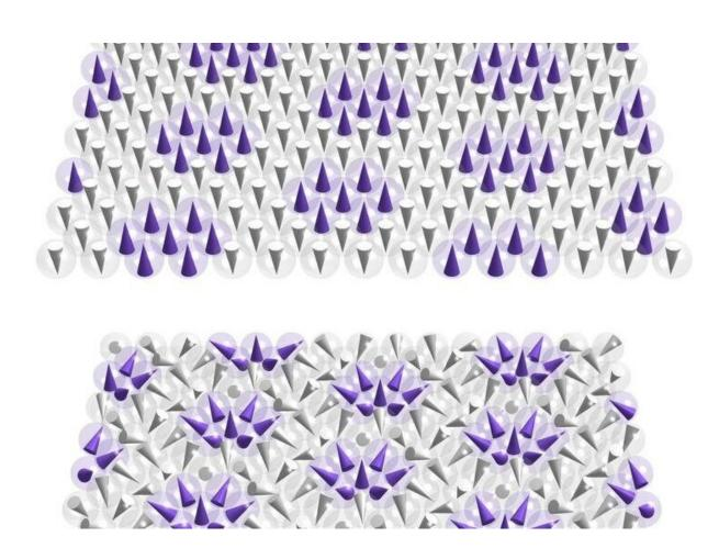
The different orientation of atomic bar magnets of an iron film: In a magnetic mosaic lattice (above), they are oriented in groups either upwards (purple) or downwards (white). In the skyrmion lattice (below), they point in all directions. Credit: André Kubetzka
