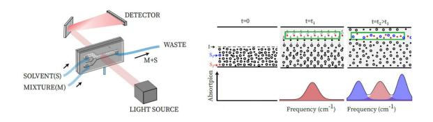
Schematic representation of the IR-DOSY setup (left) and its operation (right). A sample solution (M) and pure solvent (S) are pumped into a channel (4 mm wide). The flow rates of the sample solution and solvent are the same, so at the midpoint of the channel an interface I establishes. When measuring the IR absorption in the solvent-filled half (the green bordered region), a time-
