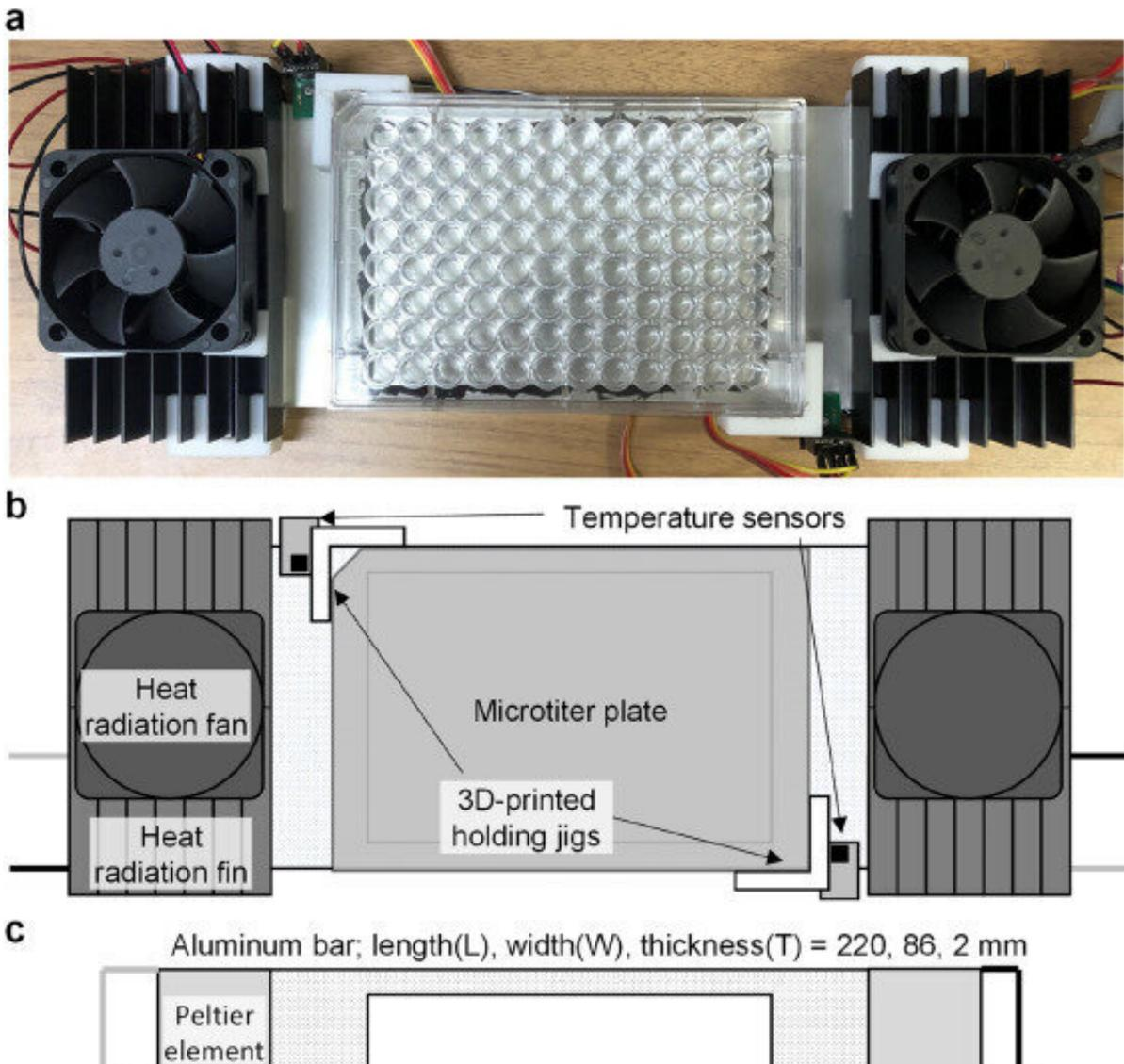
Overview of temperature gradient devices. (a, b) The device holds a microtiter plate at the center of a base aluminum plate (dotted plane in b and c) with 3D-printed jigs. The device has a temperature sensor beside two corners of the
