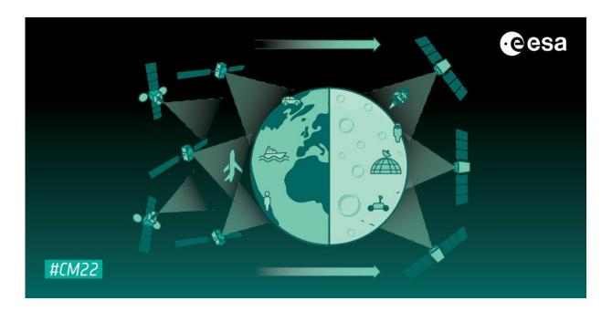
A vision of future, layered, satellite navigation, stretching from Earth to the Moon. Galileo satellites in medium Earth orbit and EGNOS augmentation satellites in geostationary orbit are supplemented by additional navigation satellites in low Earth orbit, providing stronger signals in additional frequency bands, as well as Moonlight satellites in orbit around the Moon, extending satnav coverage (as well as telecommunications links) to our natural satellite. Credit: ESA
