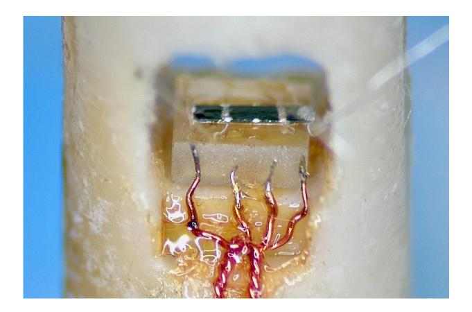
The sample holder that was used for high field measurements at Toulouse. The length of the black single crystal sample is less than 2 mm, the contacts were made with silver epoxy and 25 micrometer wires, and the sample is mounted on a sapphire plate Credit: Ataei M.Sc. thesis https://savoirs.usherbrooke.ca/handle/11143/15285
