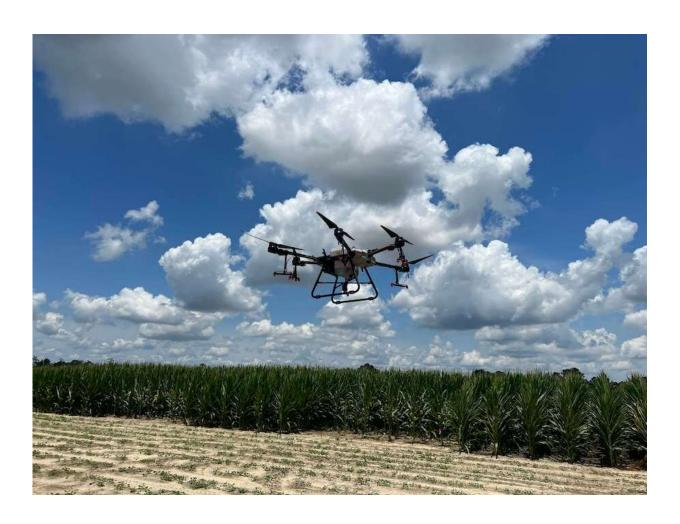
When properly programmed and operated, sprayer drones are able to fly above crops to apply chemicals using a small tank and spray nozzles, avoiding muddy fields and difficult terrain, all while providing the targeted application that saves growers money and time. Credit: Simer Virk
