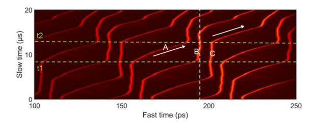
At moment t1, soliton A moves close to the soliton molecule consisted of soliton B and C; at moment t2, soliton A elastically collides with the soliton molecule: soliton A exchanges both the energy and momentum with soliton C through soliton B. After collision, soliton A together with soliton B form a new soliton molecule and soliton C leaves the new soliton molecule at the original speed of soliton A. Credit: *Light: Science & Applications* (2022). DOI: 10.1038/s41377-022-00986-3
