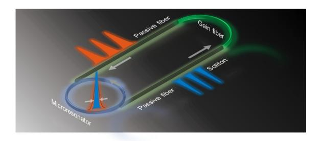
A passive nonlinear microresonator is nested in an active fiber laser cavity. Self-starting soliton microcomb with low noise, high mode efficiency, and high output power was demonstrated. Intriguing phenomenon such as soliton Newton's cradle was observed with an ultrafast time magnifier for the first time. Credit: *Light: Science & Applications* (2022). DOI: 10.1038/s41377-022-00986-3
