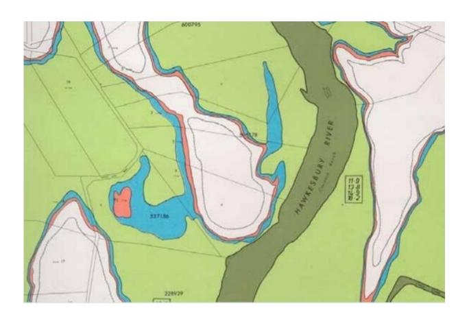
Paper flood maps such as this extract from the 1982 Lower Hawkesbury Floodplain Atlas, do not include critical details such as water depth, velocity, rate of rise and potential isolation. Author provided
