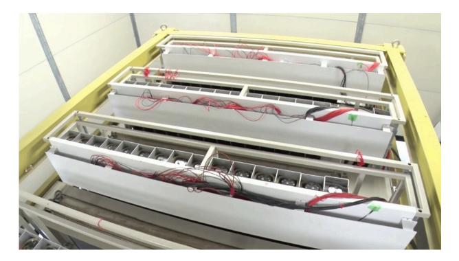
These are the sensors used to detect the weakly interacting muon particles. Each scintillator sensor is extremely dense to maximize the chances that a muon will interact with it. Arranged in a grid, the sensors can form a crude image of whatever the muons passed through to reach the sensor. Credit: ©2022 Hiroyuki KM Tanaka
