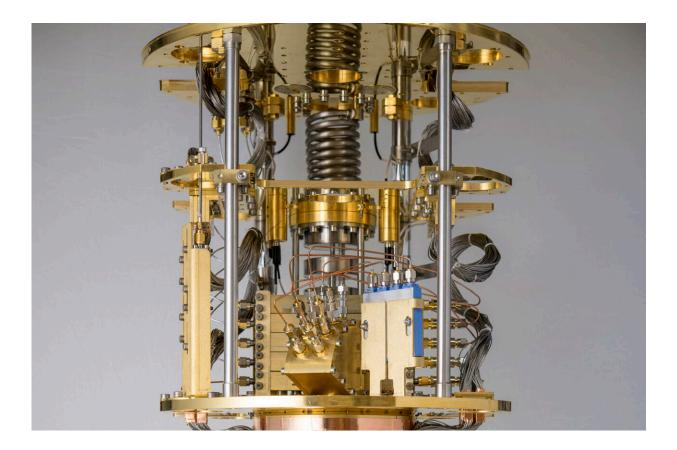
D-Wave quantum annealing processors use thousands of superconducting flux qubits on a lithographed chip, suspended in an environment near absolute zero. Credit: D-Wave.
