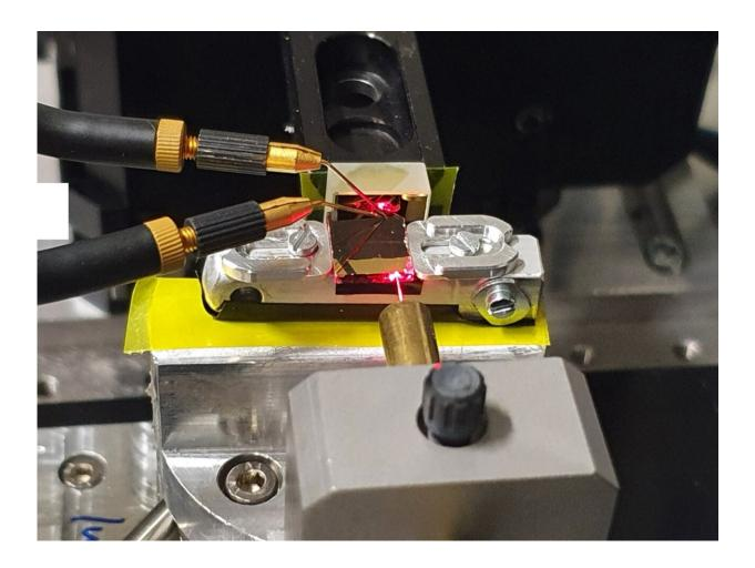
The experimental setup: A red alignment laser was used to visualize the beam path from the fiber into the optical waveguide and its reflection at a gold mirror. Two microprobes were used to contact the photoconductor, the size of which is in the subwavelength range. Credit: Empa
