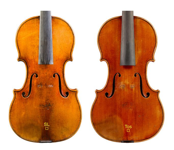
A highly precise, nanometer-scale imaging technique revealed a protein-based layer between the wood and the varnish coating of these two Stradivarius violins. Credit: Adapted from *Analytical Chemistry* (2022). DOI:
