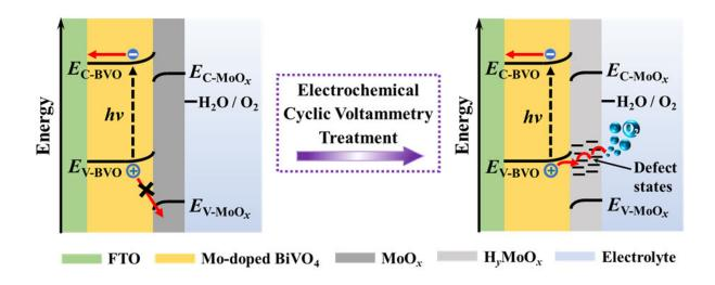
Electrochemical cyclic voltammetry treatment initiates the formation of HyMoOx surface defects, which act as charge transfer channels for photogenerated holes. Via these charge transfer channels, the charge separation and photoelectrochemical performance of Mo-doped BiVO4 electrode are significantly enhanced. Credit: *Chinese Journal of Catalysis* (2022). DOI: 10.1016/S1872-2067(21)63986-4
