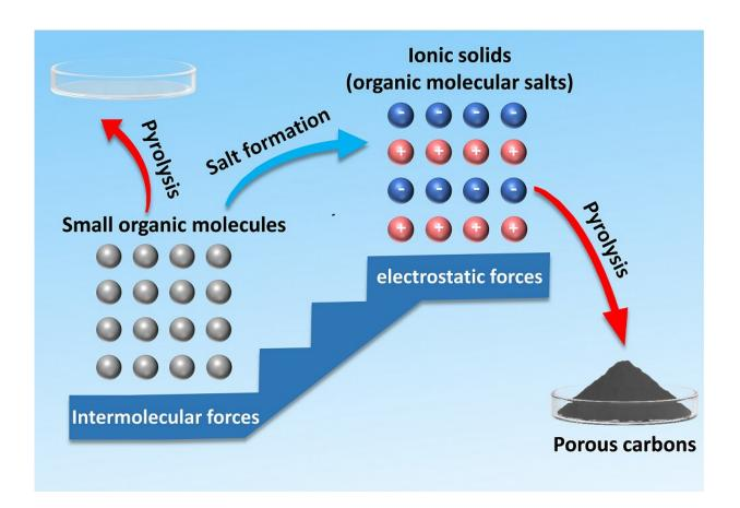
This graphic shows how small organic molecules can be transformed into organic molecular salts, or ionic solids. The organic molecular salts can then be transformed into porous carbons through pyrolysis, which is using high temperatures to activate a transformation. Porous carbons are essential for creating carbon nanostructures, which can be used in a variety of industries. Credit: *Nano Research*
