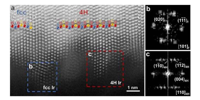
(a) Aberration-corrected HAADF-STEM image of Au@4H/fcc-Ir0.14 nanostructures. (b,c) FFT patterns of the corresponding regions marked with blue (b) and red (c) dashed squares in a. Credit: *Proceedings of the National Academy of Sciences* (2022). DOI: 10.1073/pnas.2204666119
