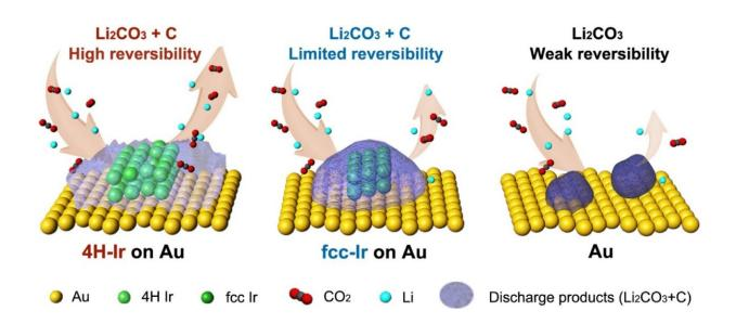
Three different kinds of electrochemical reaction kinetics on Au@4H-Ir, Au@fcc-Ir and pure Au (right panel) in an aprotic Li-CO<sub>2</sub> battery. Credit: *Proceedings of the National Academy of Sciences* (2022). DOI: 10.1073/pnas.2204666119
