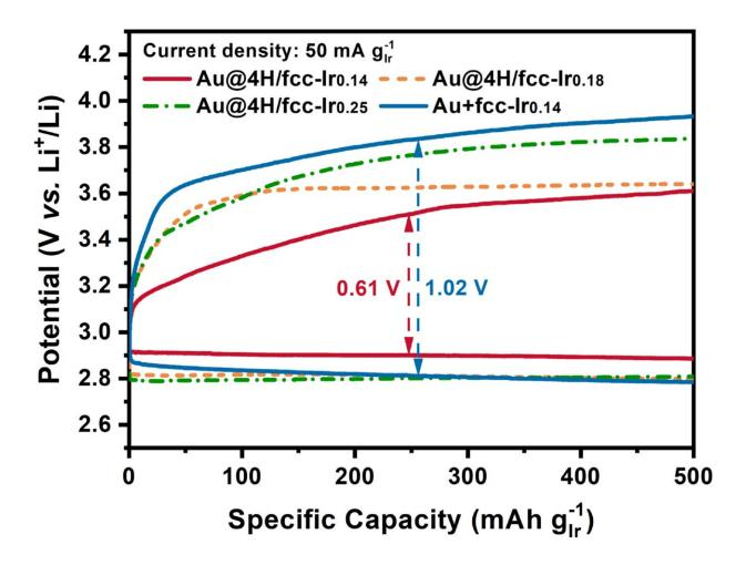
Discharge-charge profiles of as-prepared Au@4H/fcc-Irx and Au+fcc-Ir0.14 cathodes in an aprotic Li-CO<sub>2</sub> battery. Credit: *Proceedings of the National Academy of Sciences* (2022). DOI: 10.1073/pnas.2204666119
