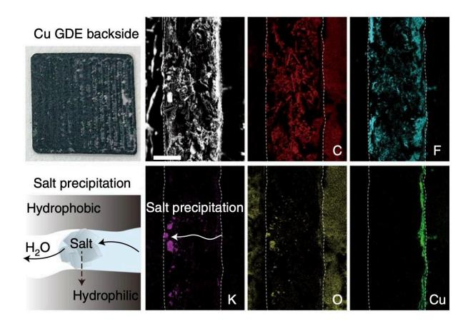
Cross-sectional scanning electron microscopy and energy-dispersive X-ray spectroscopy elemental mapping images of the Cu GDE after electrolysis, indicating the severe salt precipitation occurring in the hydrophobic pores of Cu GDE. Scale bar, 100  $\mu$ m. Credit: Li et al. (*Nature Energy*, 2022)
