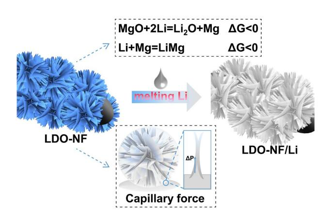
Interfacial reaction driving force together with capillary force facilitate the transient infiltration of molten Li into a 3D host for stable 3D composite lithium anode. Credit: *Nano Research* (2022). DOI: 10.1007/s12274-022-4981-3
