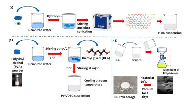
Schematics of the fabrication process of BN-PVA aerogels. Credit: *Polymers* (2022). DOI: 10.3390/polym14163316
