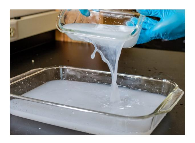
Dr. Jiang's process breaks down wood fibers (sourced from forest waste) in a solution of cold sodium hydroxide combined with mild mechanical blending. Credit: University of British Columbia
