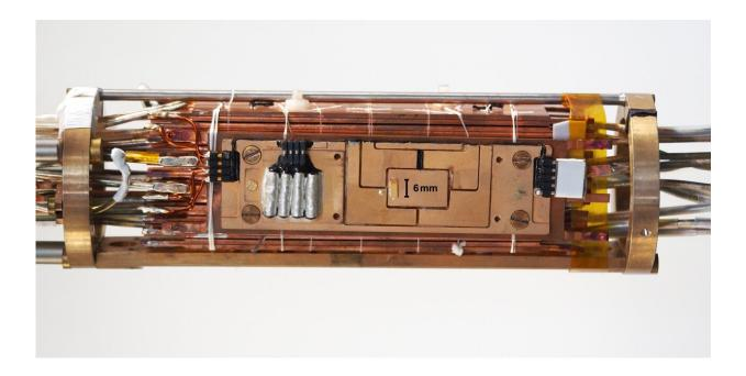
The cryostat used by the Basel physicists to reach a record temperature of 220 micro-Kelvin. The special thermometer along with a scale bar can be seen in the center of the image (golden rectangle). Credit: University of Basel, Department of Physics
