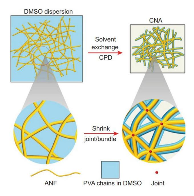
Schematics of the assembly process of the composite nanofiber aerogels. Credit: The University of Hong Kong
