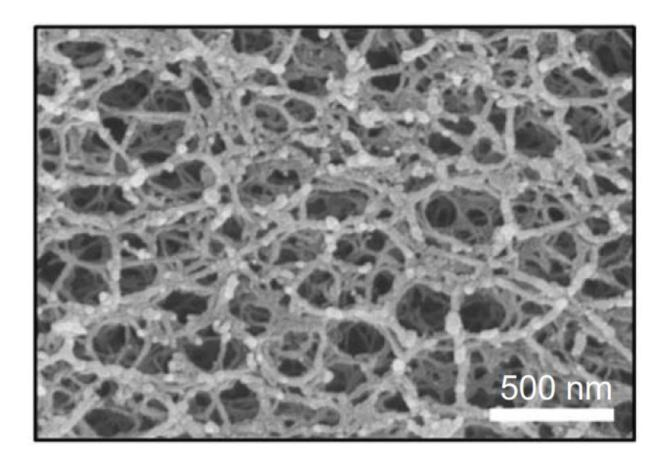
Scanning electron microscope image showing the micro-structure of the aerogel materials. Credit: The University of Hong Kong
