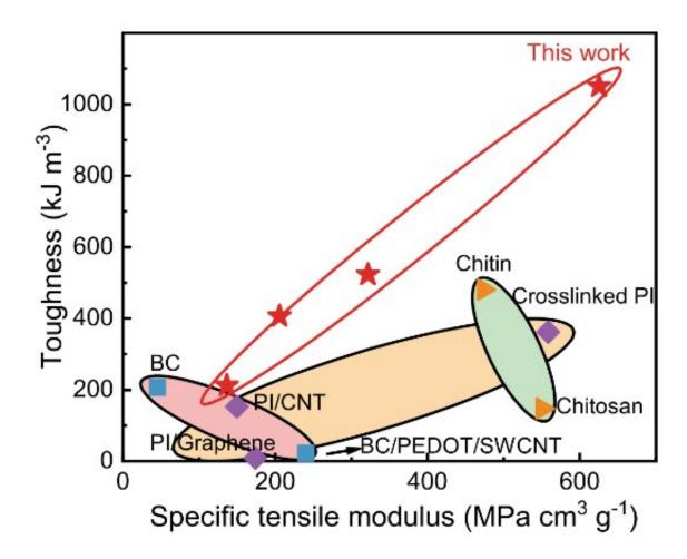
Both high toughness and tensile modulus are achieved by the composite nanofiber aerogels, when compared to other polymeric aerogels. Credit: The University of Hong Kong
