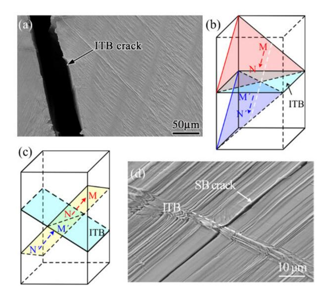
Fatigue damage behavior of ITB in copper bicrystal at different angles to the loading axis. (a,b) ITB is perpendicular to the loading axis; (c,d) ITB inclines to the loading axis. Credit: IMR
