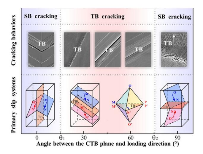
Fatigue damage mechanisms corresponding to different inclination angles of CTB and loading axis of copper bicrystal. Credit: IMR
