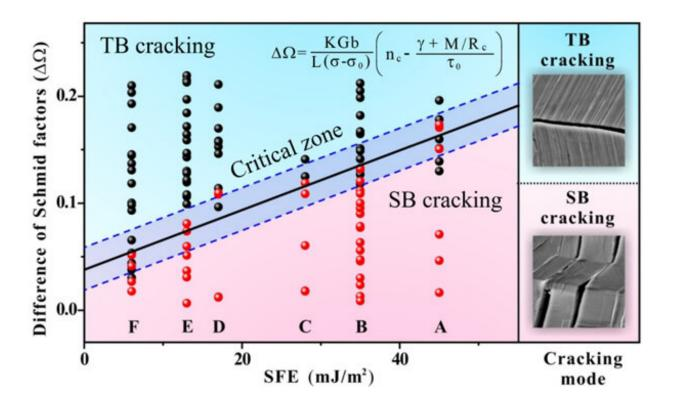
Synergistic effect of stacking fault energy and crystal orientation on the fatigue cracking behavior of polycrystal copper alloy. Credit: IMR
