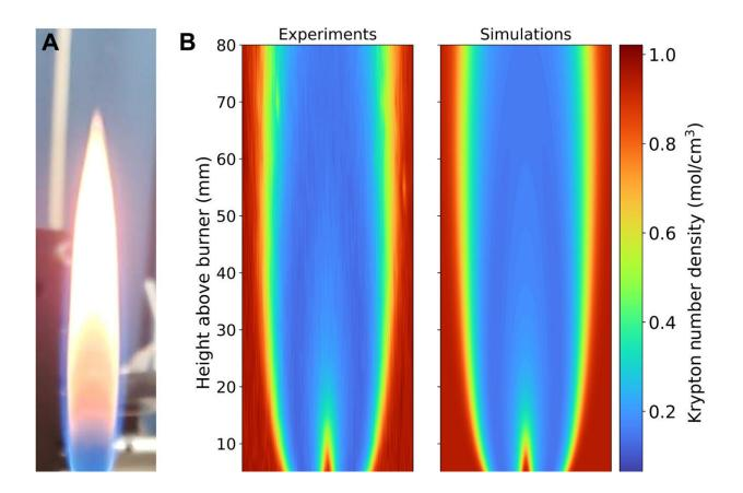
Measured and simulated krypton number densities in a sooting methane/air flame. (A) A photograph of the flame sized to the same spatial scale as (B). (B) Image plots of experimental (left) and simulated (right) krypton number densities throughout the flame. (C) Radial profiles of krypton number density at several heights above burner (HABs). Error bars for the measurements are represented by gray-shaded regions. Total time to collect 2D data: 2 hours.
