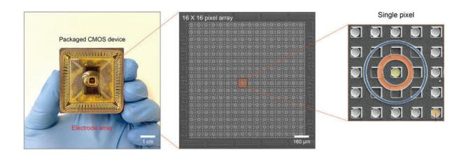
A CMOS chip (left) with an array (center) of hundreds of individual ionic transistors (right). Credit: Woo-Bin Jung/Harvard SEAS
