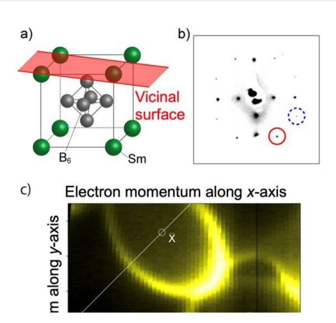
Fig. 1 (a) Crystal structure of SmB6 and the vicinal surface used in this study. (b) Obtained electron diffraction pattern of the anisotropic surface superstructure.
