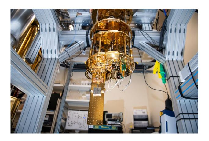
A superconducting qubit sits in a dilution refrigerator in a Pacific Northwest National Laboratory (PNNL) physics lab. This experimental device is the first step in establishing a qubit testbed at PNNL. Credit: Andrea Starr | Pacific Northwest National Laboratory
