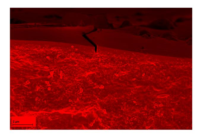
The SEM images show the cross-sections of NBR and SBR elastomers exposed to the He + ion beam with a fluency of  $1 \times 10^{17}$  cm-2.Irradiation with a highenergy ion beam causes cross-linking of the polymer surface layer. The core of the non-ionized material remains flexible and can stretch the rigid top layer, causing the surface layer to wrinkle and micro-crack. Credit: NCBJ
