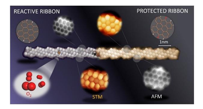
Scanning probe microscopy image of a reactive (left) and protected (right) graphene nanoribbon. Credit: DIPC | CFM | FZU | CiQUS | CATRIN
