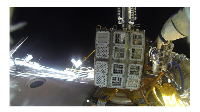
EXPOSE-R2 platform outside of the ISS with BIOMEX experiment. Credit: Roscomos/ESA
