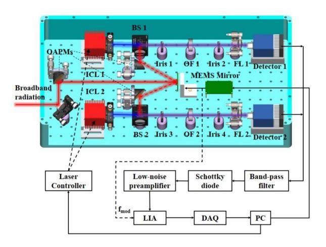
Schematic diagram of the experimental setup. Credit: Xue Zhenyue
