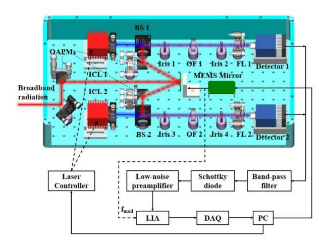
Schematic diagram of the experimental setup. Credit: Xue Zhenyue
