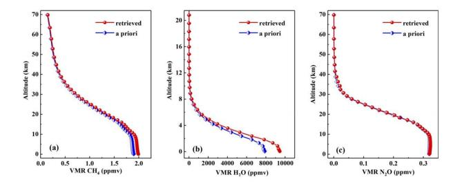
The retrieved vertical concentration profiles of (a)  $CH_4$ , (b) water vapor and (c)  $N_2O$ . Credit: Xue Zhenyue
