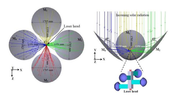
Simplified scheme of a side-pumped solar laser system with four off-axis parabolic mirrors: (left) front view and (right) side view; (inset) laser head is mounted at the common center point of the four off-axis parabolic mirrors. Credit: Rabeh Boutaka et al, *Journal of Photonics for Energy* (2022). DOI: 10.1117/1.JPE.12.038002
