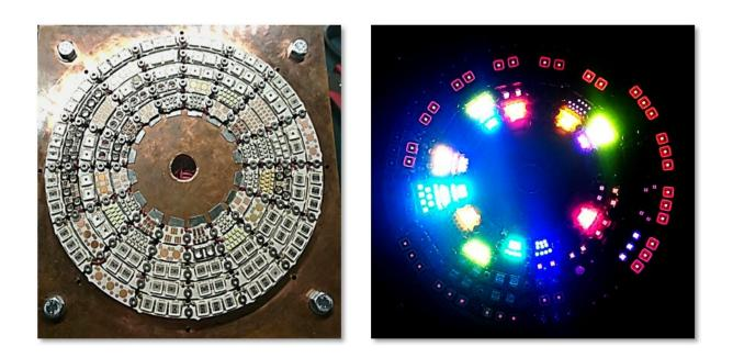
The Star Light Simulator (left) and illuminated (right). It has 25 channels total, emitting light from 365 nanometres (UV light) to 940 nanometres (infrared light). Credit: La Rocca et al.
