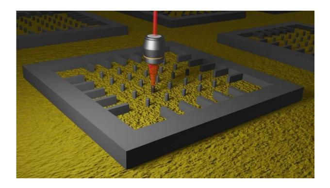
The researchers use an objective lens to test the light output from an array of silicon nanopillars on a chip. Credit: HZDR / Juan Baratech
