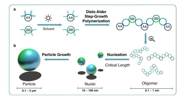
Principle of light induced particle formation. a Under irradiation, an AA monomer forms a reactive intermediate, which reacts with a BB monomer in a Diels-Alder step-growth polymerization. b As the linear polymer chains grow, they precipitate from solution to form particles. Credit: *Nature Communications* (2022). DOI: 10.1038/s41467-022-32429-3
